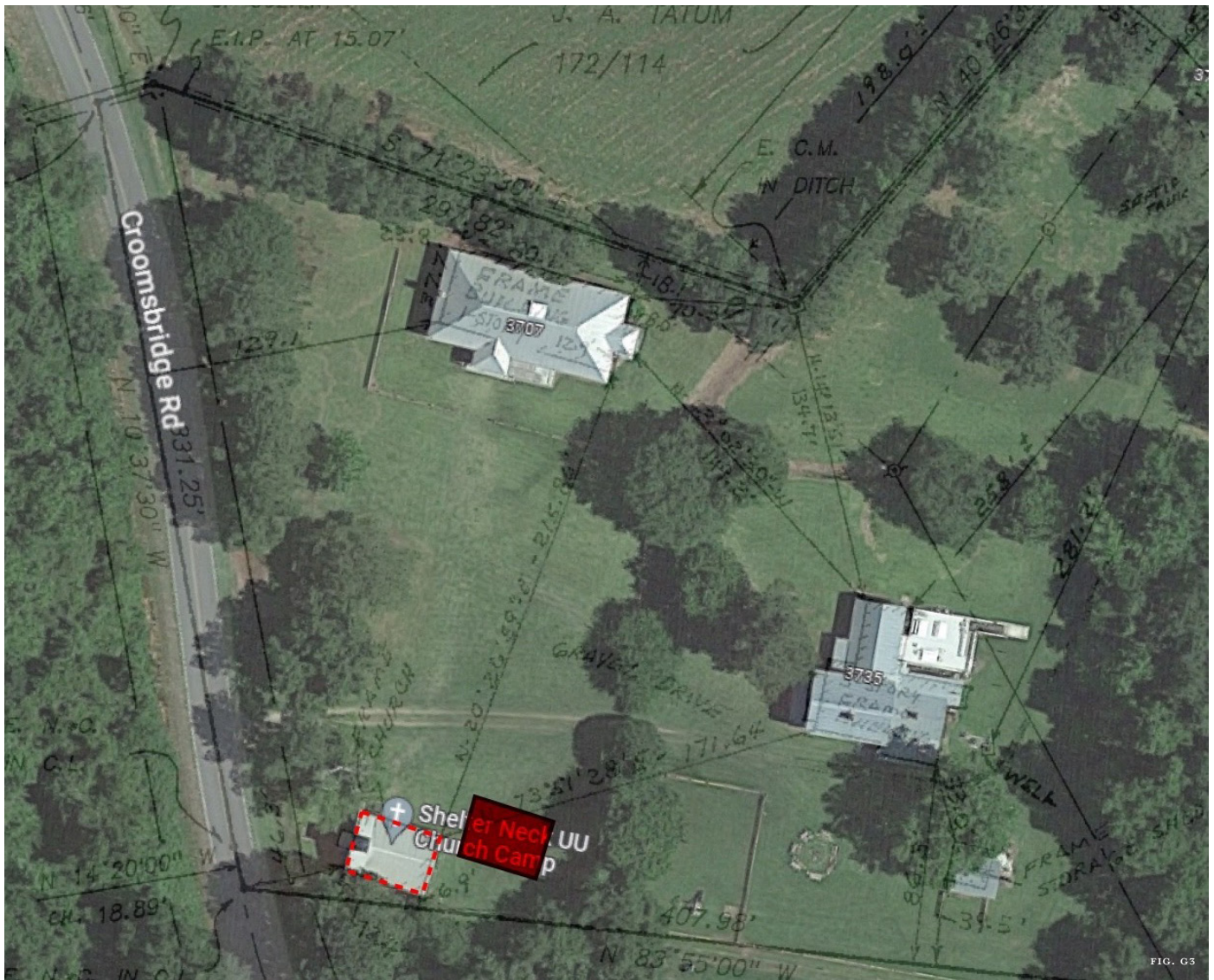
Figure G3: To elevate all three Shelter Neck UU Camp (formerly, Carolina Industrial School) buildings in Pender County at least 6 feet, a combination of strategies has been proposed to mitigate the increased elevation while maintaining the buildings' historic integrity: increase the height of the foundation walls, install retaining walls 10–15 feet away from each building's footprint, add fill that slopes from the foundations to the retaining walls, and screen the foundation walls with vegetation.
